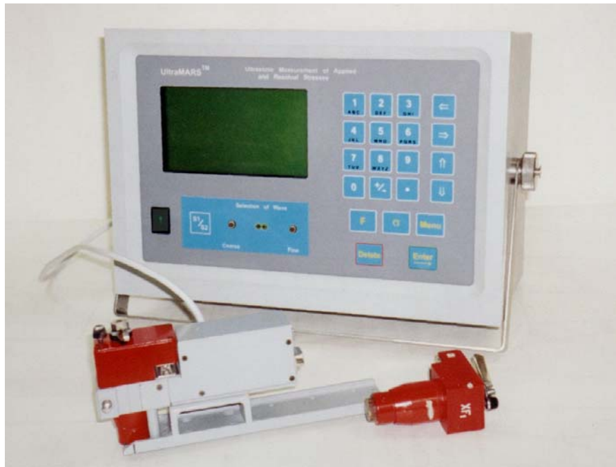
Figure 2. The developed device with sensors for ultrasonic measurement of residual stresses
