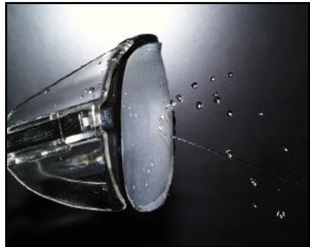
Lens laminated with the super-hydrophobic film
