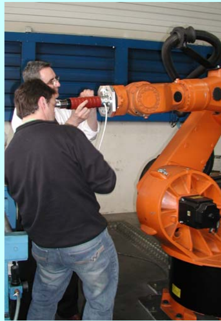
Installation by ITL engineers of a robotic version of the UltraPeen™ instrument onto a robot.
