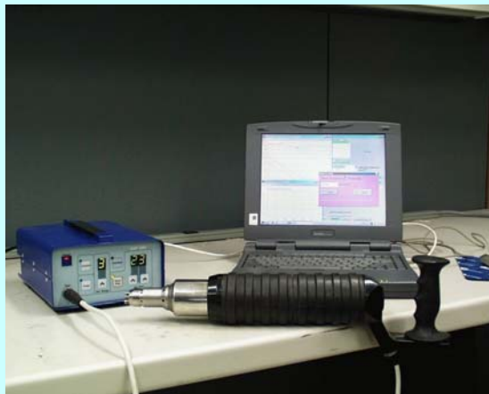
Manual UP instrument UltraPeen™ (shown with an optional laptop computer)
