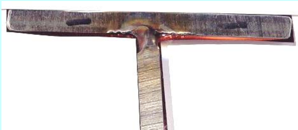
T-welded two 6 mm steel plates: after UP treatment
