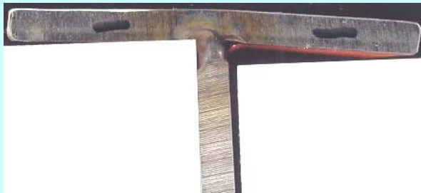
T-welded two 6 mm steel plates: before UP treatment
