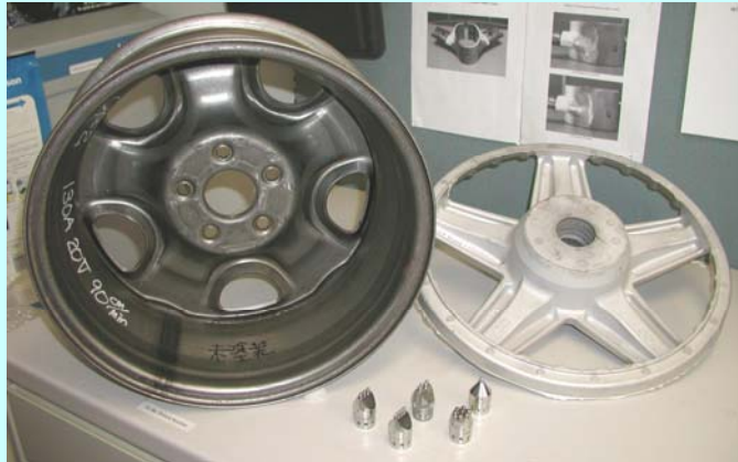
Steel welded wheel and aluminum wheel improved by Ultrasonic Peening
