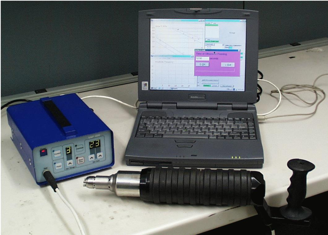
Figure 10. Computerized Complex for Ultrasonic Peening of parts and welded elements
