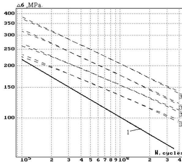
Figure 2. Fatigue curves of non-load-carrying fillet welded joint:
