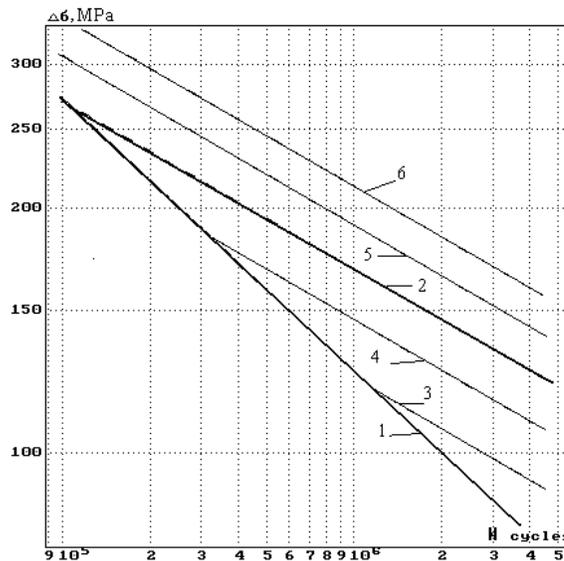
Figure 1. Fatigue curves of transverse loaded butt weld at  $R=0$ :
