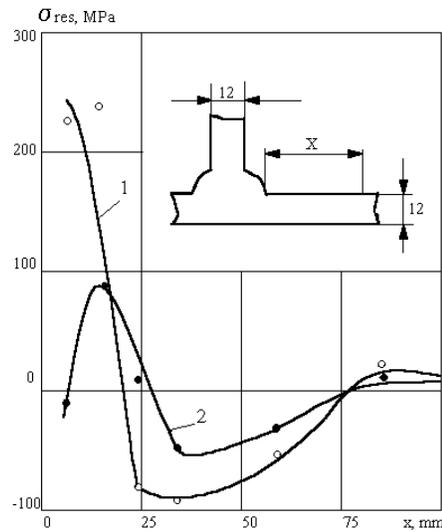
FIGURE 3. Distribution of residual stresses near the fillet weld in the railway bridge span:
