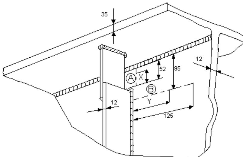
FIGURE 2. Fragment of the railway welded bridge span:
